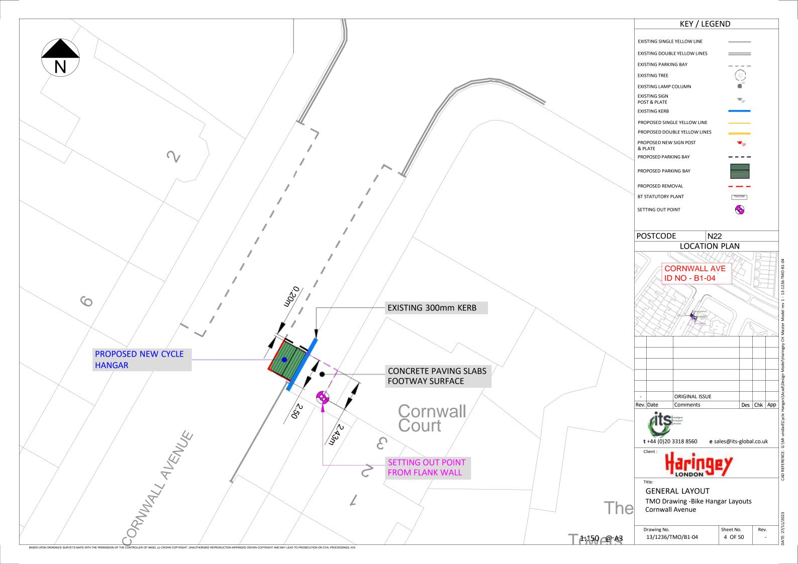
**EXISTING SINGLE YELLOW LINE EXISTING DOUBLE YELLOW LINES** EXISTING TREE **EXISTING SIGN** POST & PLATE EXISTING KERB & PLATE PROPOSED NEW CYCLE **HANGAR** 0.20m EXISTING 150mm KERB 5.78m NIGHTINGALE ROAD **ASPHALT FOOTWAY** SP 2.50m **SURFACE** SETTING OUT POINT FROM **EDGE OF PLANTER SURFACE** 4.46m 69 Rev. Date
